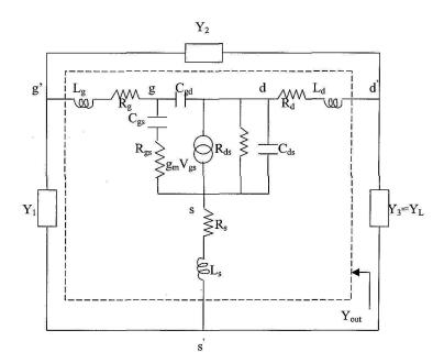
Figure 2 Parallel feedback topology for a MESFET oscillator.
