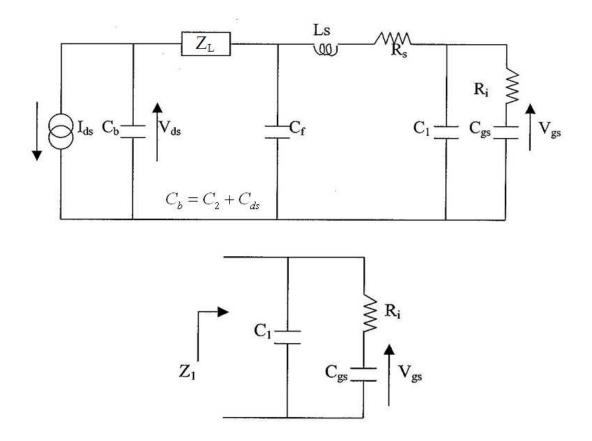
Figure 6 An equivalent circuit of the open loop model of a MESFET oscillator.
