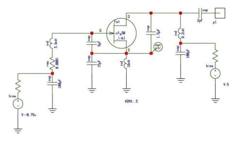
Figure 10 Schematic of the test oscillator based on [1].
