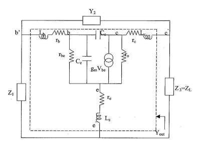
Figure 4 A parallel feedback topology of an oscillator using a bipolar transistor.
