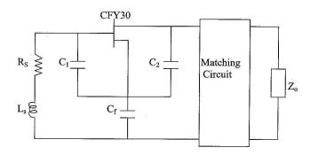
Figure 5 A 950 MHz MESFET oscillator circuit configuration.
