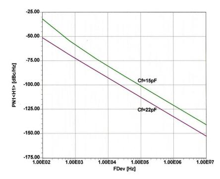
Figure 14 Simulated and validated noise figure of the circuit shown in Figure 10. An increase of the feedback capacitor from 15 to 22pF improves the phase noise.
