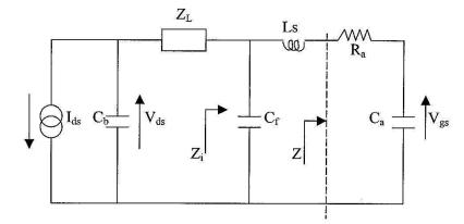
Figure 7 A simplified open loop model of the oscillator.
